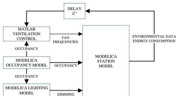
Figure 1. The Modelica Model-in-the-loop simulator
