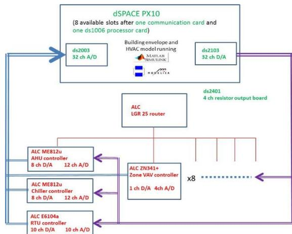
Figure 3. Schematic of HiL setup.
