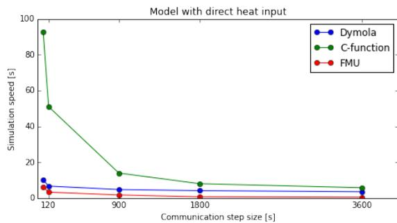
Figure 3: Simulation speed for the different cosimulation methods for the detailed building.
