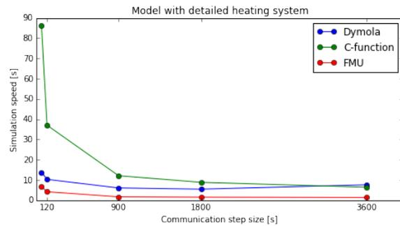
Figure 4: Simulation speed for the different co-simulation methods for the detailed building model with heating system.
