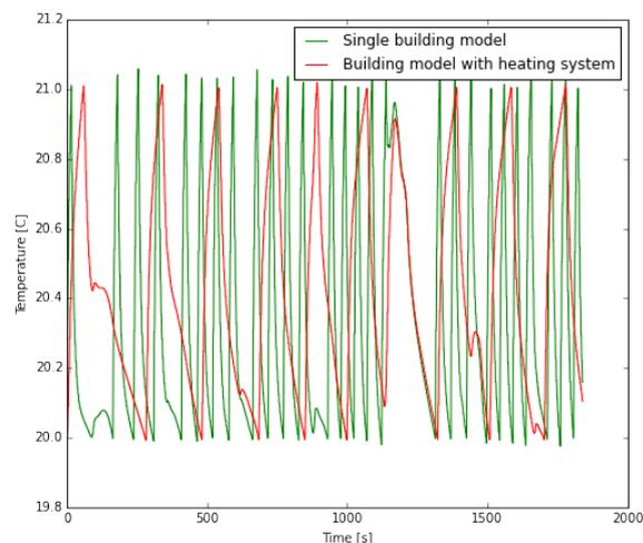
Figure 1: Response of a single building model (green) and building model with heating system (red) to a hysteresis control input.
