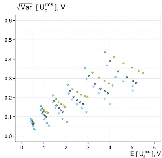
Figure 5: Standard deviation of the aleatory uncertainty of the characteristic voltage deviation  $U_{\phi}^{rms}$  in the low-voltage feeder by occupant behaviour regarding six different feeder sizes and five degrees of implementation of heat pump and photovoltaic based building energy systems (redrawn from Baetens and Saelens (2015)).
