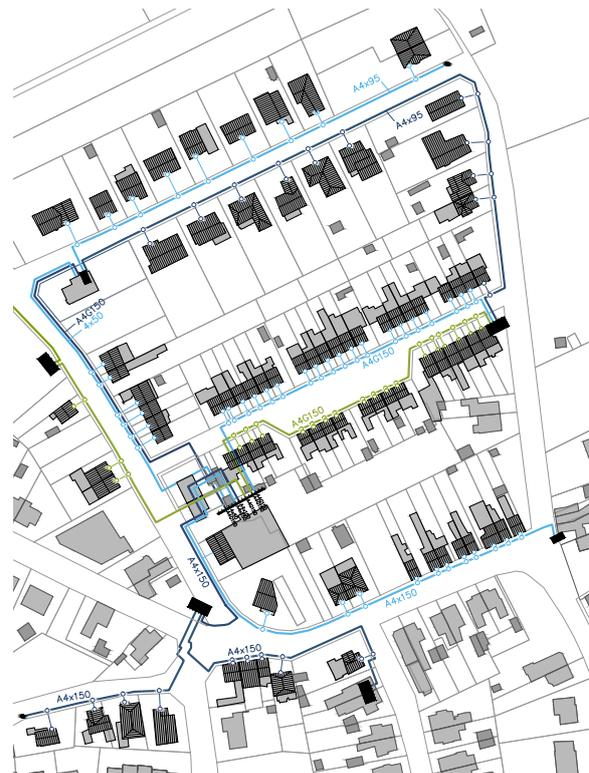
Figure 1: Graphical representation of an example low-voltage distribution island connecting 85 dwellings by seven radial three-phase feeders to a 10/0.4 kV transformer with a nominal capacity of 250 kVA.
