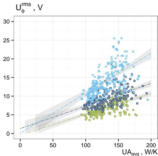
Figure 4: Correlation between the average UA-value of heat pump based dwellings on the characteristic daily voltage deviation  $U_{\phi}^{rms}$  in the low-voltage feeder regarding three feeder strengths (redrawn from Protopadaki et al. (2015)). Denoted with 'x' are the infeasible building solutions regarding distribution grid regulations.
