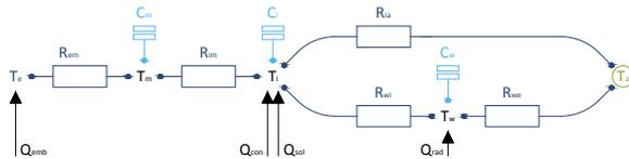
Figure 3: Example of a third-order thermal zone model in the FastBuildings library
