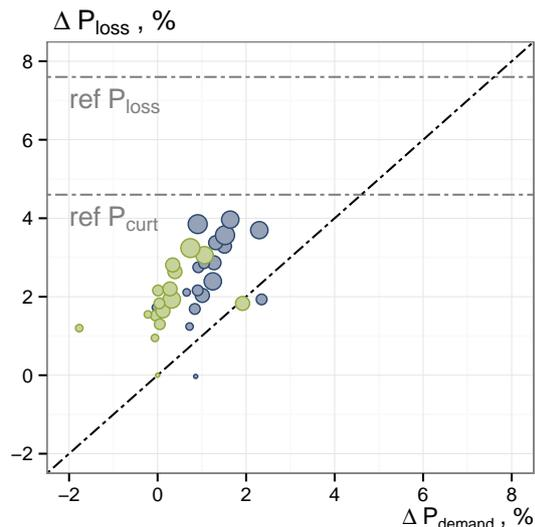
Figure 6: Loss-benefit space of the rule-based controls of the heat pump aiming to reduce the ohmic and curtailing losses with a 200 liter (green) and 500 liter hot water storage tank. (redrawn from De Coninck and Helsens (2015)).
