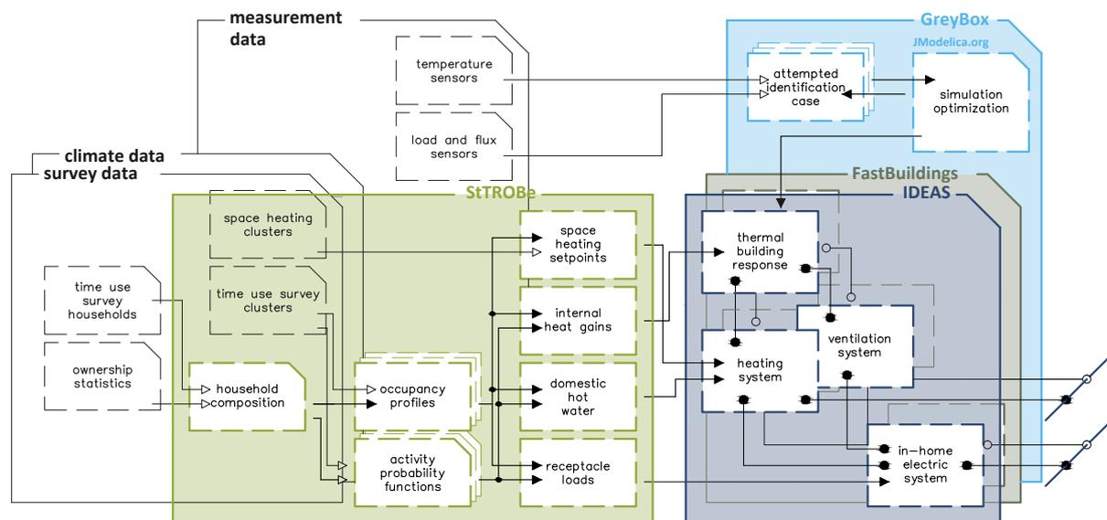
Figure 2: Overview of the OpenIDEAS Framework for integrated district energy assessments by simulation; based on IDEAS for the transient simulation of the (building and ) district energy system, on StROBe for its boundary conditions regarding stochastic occupant behaviour, and on GreyBox for generating low-order component models through system identification of measurements signal based on their implementation in FastBuildings.
